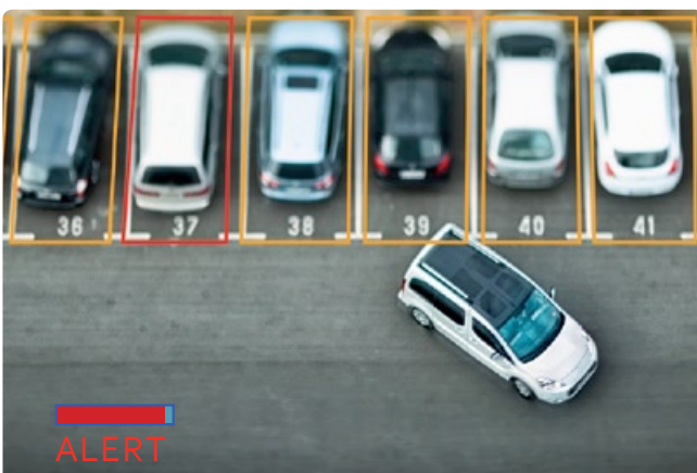
The KiwiVision ® Parking Space Analyzer alerts when the maximum parking duration is exceeded
