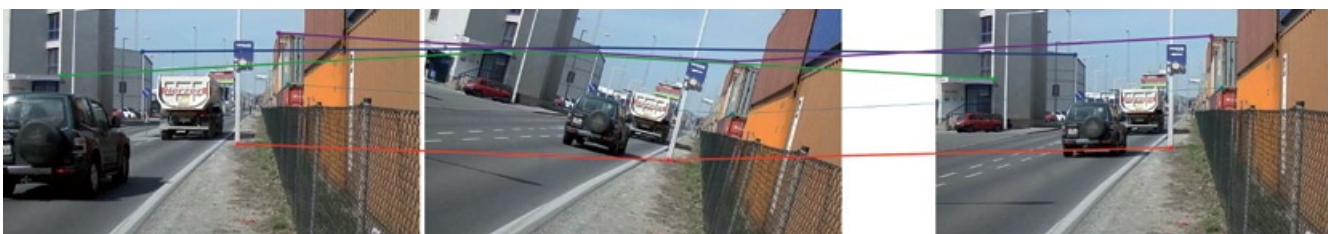
The KiwiVision ® Video Enhancer stabilizes shaking video images through the tracking of distinctive points in the video
